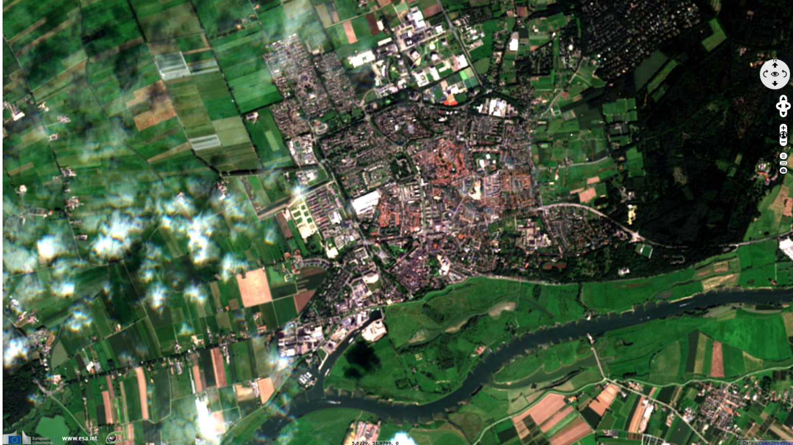
Fig. 2 - S2 MSI - NDVI with colour map - Water bodies & artificial land clearly differ from vegetated land.
