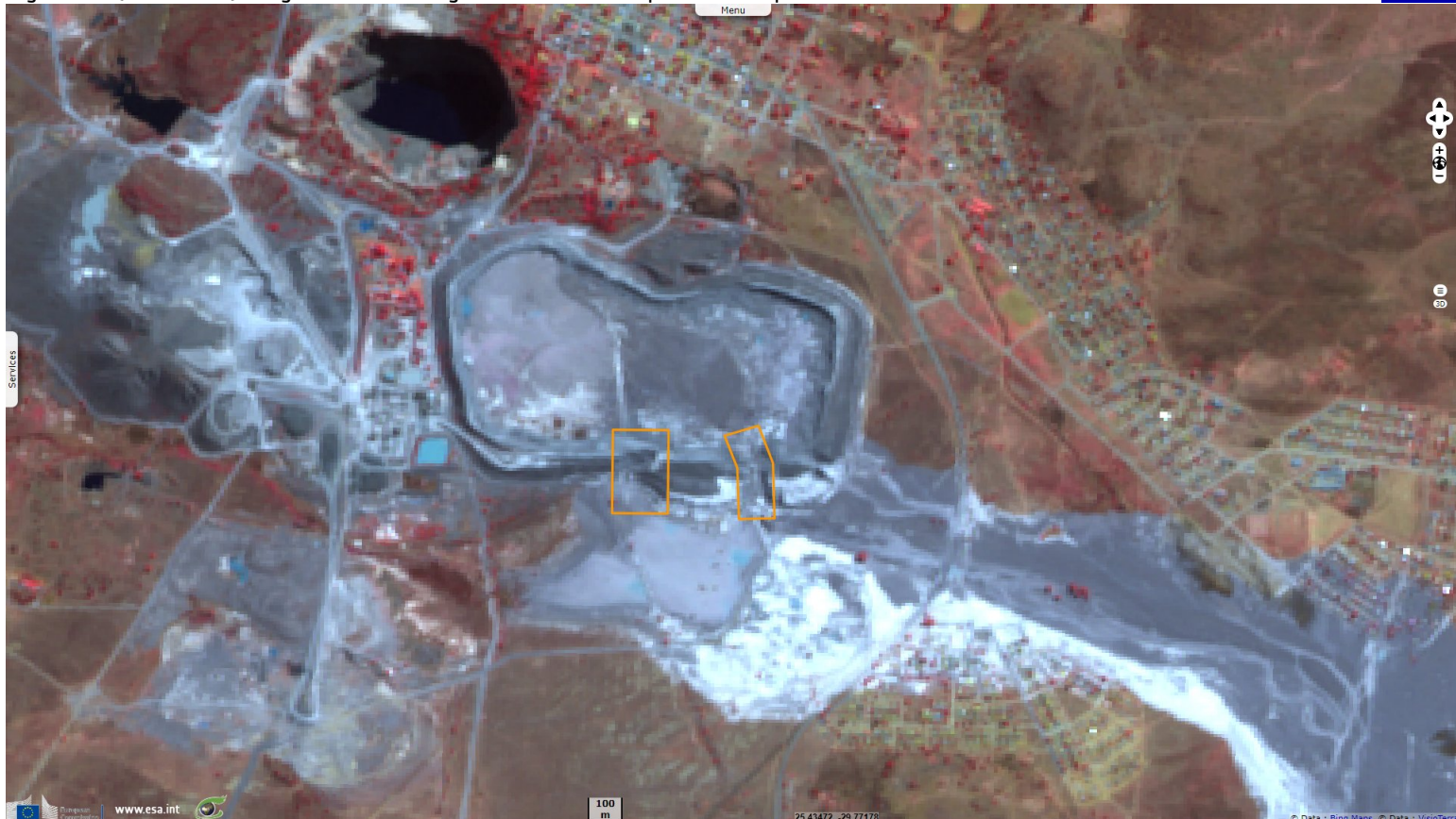
Fig. 2 - S2 (16.09.2022) - Jagersfontein mining dam after the collapse on 11 September 2022.
