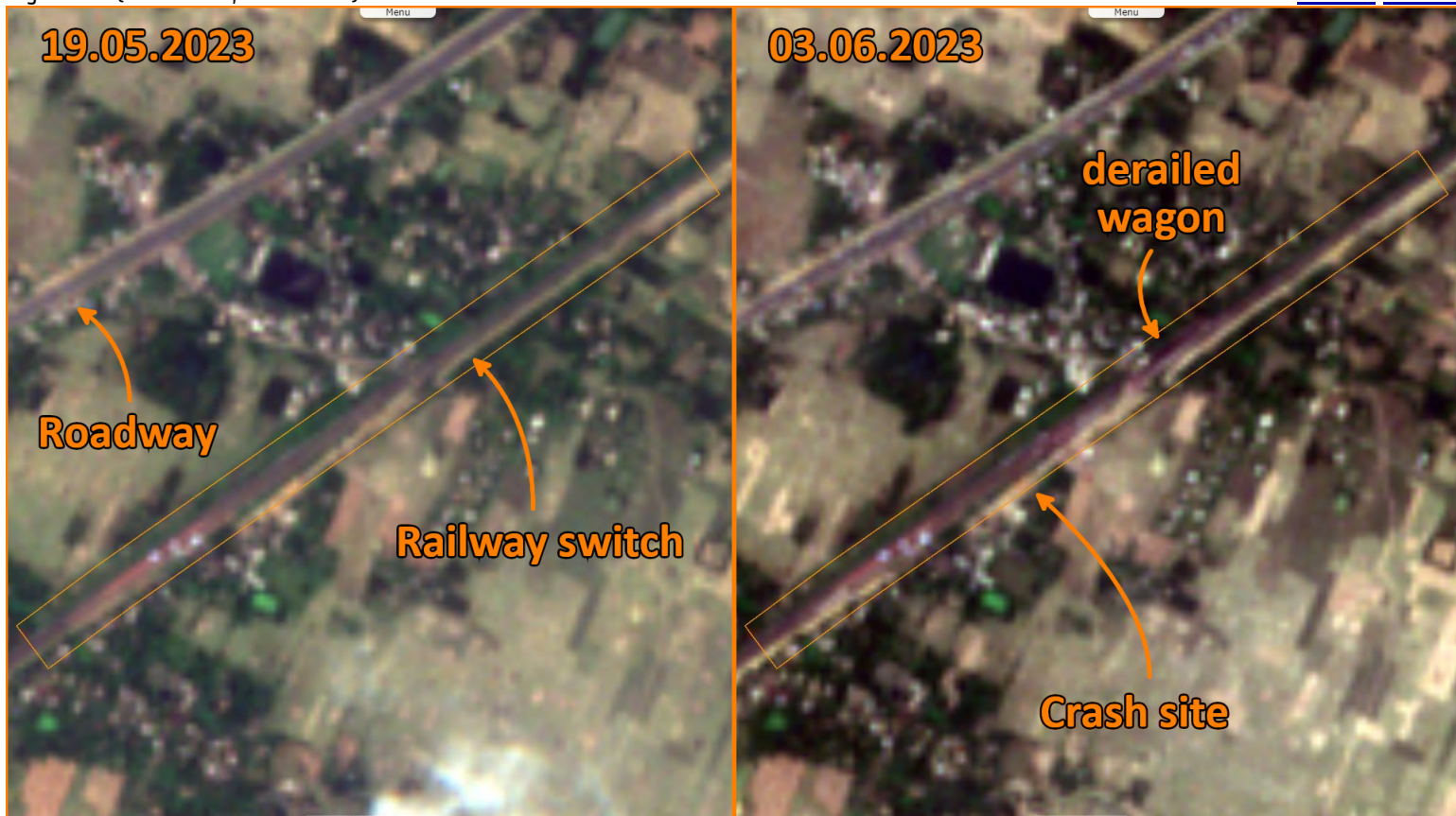
Fig. 2 - S2 (19.05.2023, 03.06.2023) - An error in a switch caused a collision between 3 trains.
