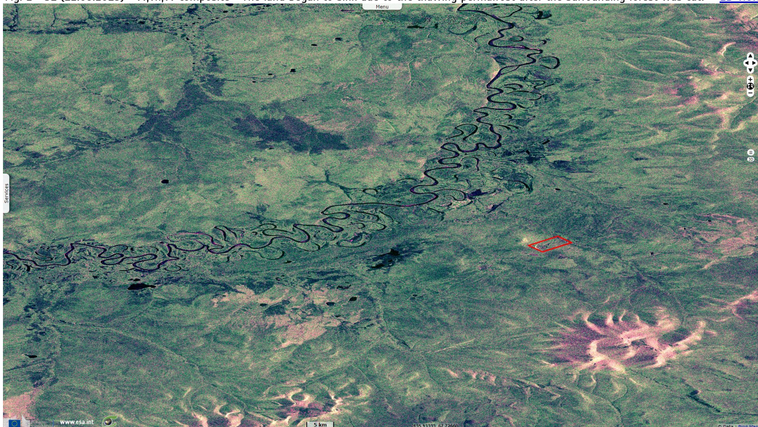
Fig. 2 - S1 (12.08.2019) - vv,vh,vv composite - The land began to sink due to the thawing permafrost after the surrounding forest was cut.
