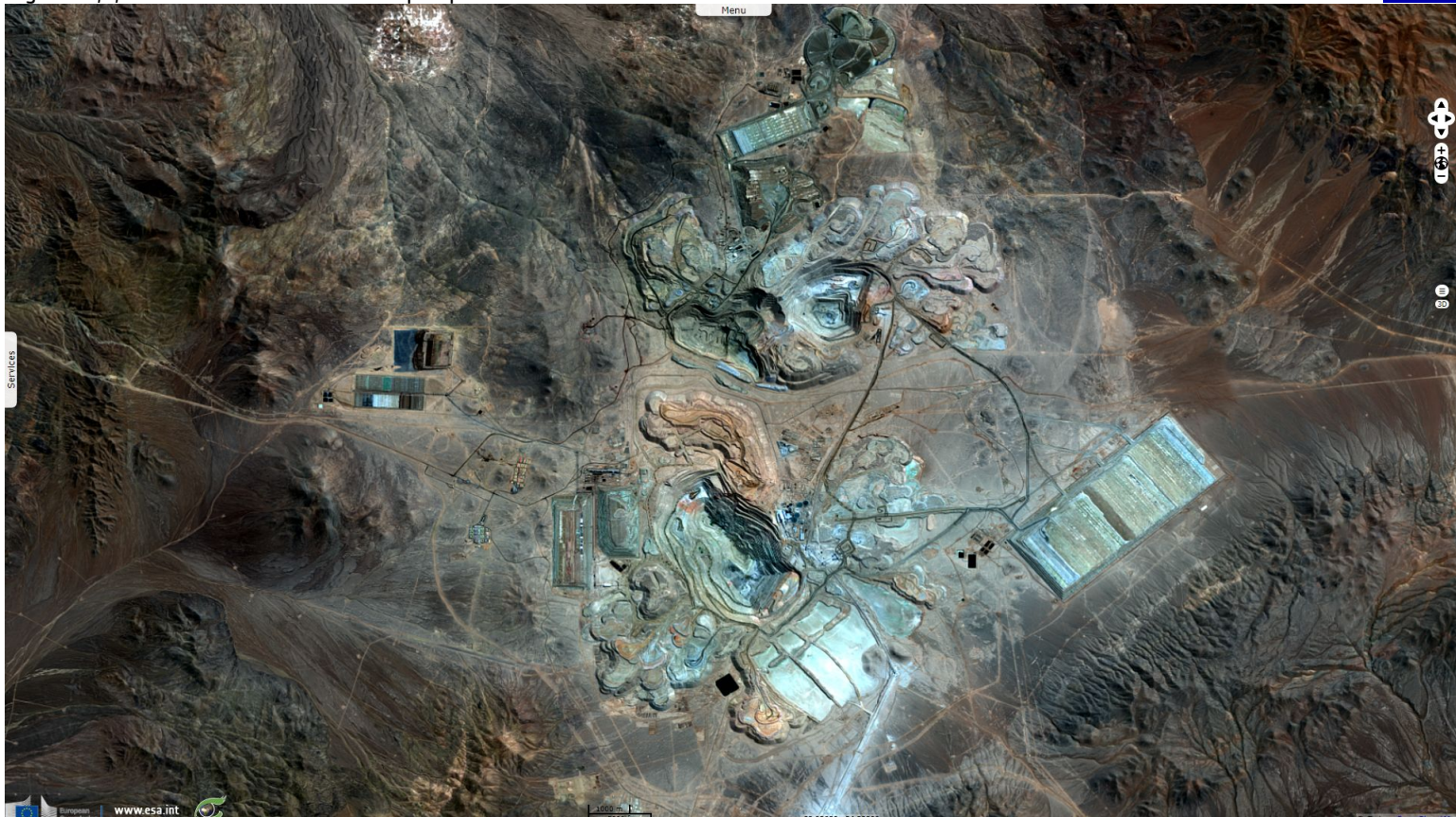
Fig. 2 - 4,3,2 natural colour - Escondida open pit shows various hues but less saturated colours in natural colour.
