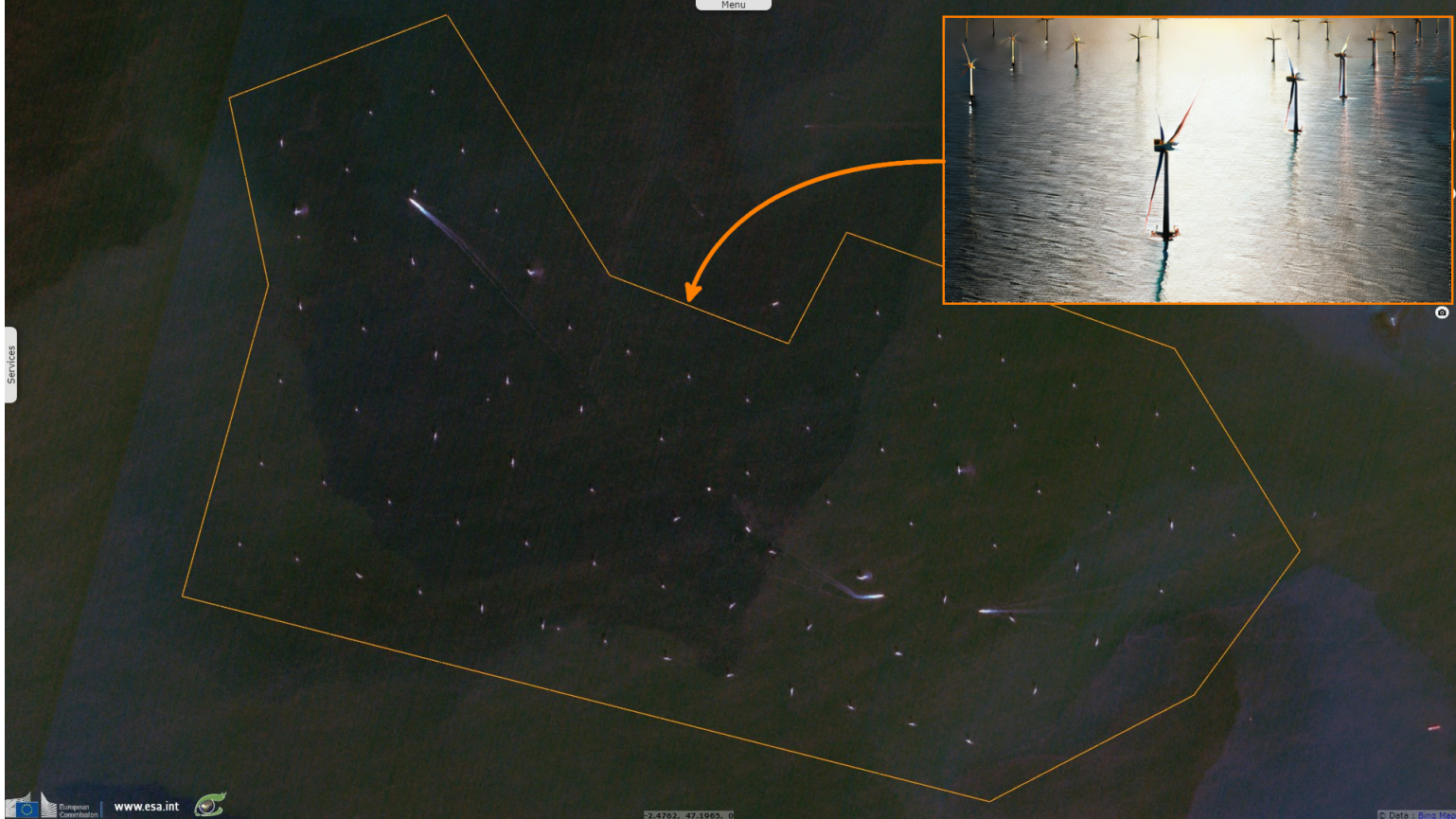
Fig. 2 - S1 (24.09.2022) - It is only the first French offshore wind farm to be connected. It has a 78 km 2 footprint for a 480 MW power. 3D view
