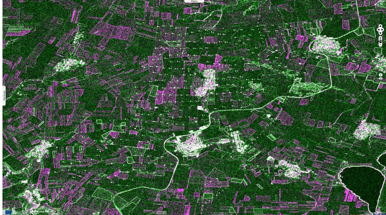
Fig. 4 - cv(vh),vh,stddev(vh) colour composite - The higher contrast computed on multitudes mean highlights turbines as pairs of dots. 2D view
