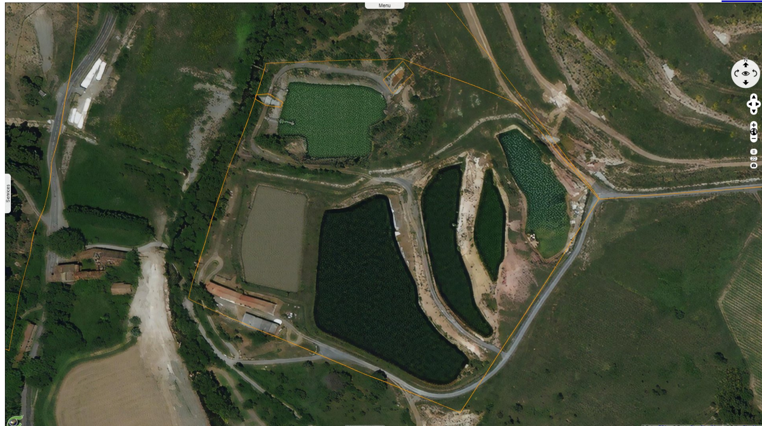
Fig. 15 - The filtration basins. The orange spot at east shows infiltrations from non watertight Artus hill. At north-west, the white trace shows arsenic overflow right into the Grésillou
