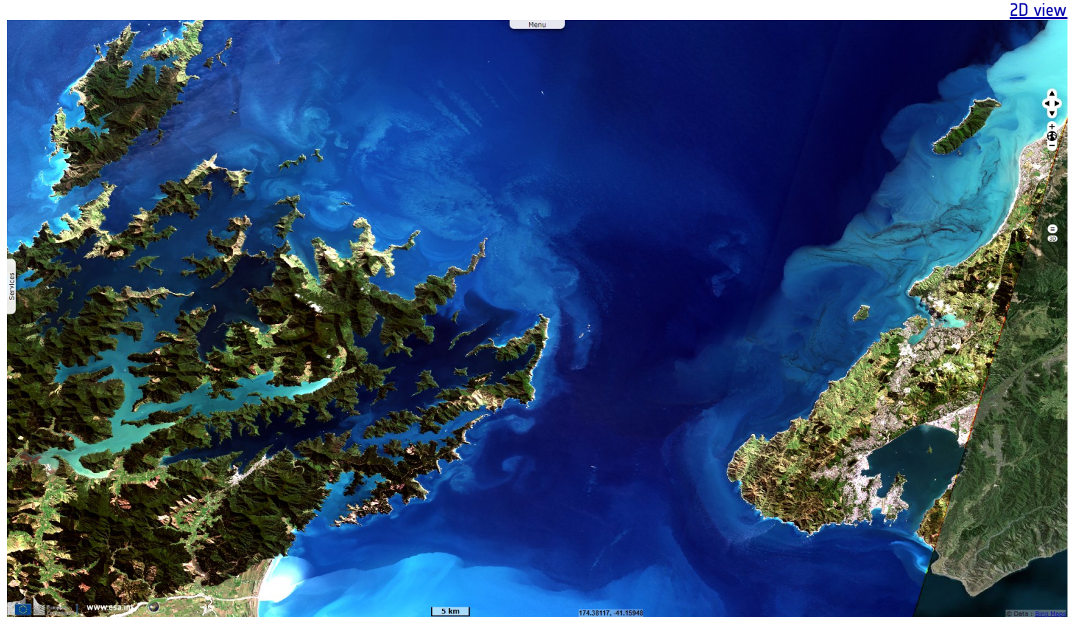
Fig. 2 - S2 (10.09.2021) - The difference in sea level can drive tidal currents up to 2.5 m/s across the strait. Despite the strong currents, there is almost zero tidal height change in the centre of the strait.
