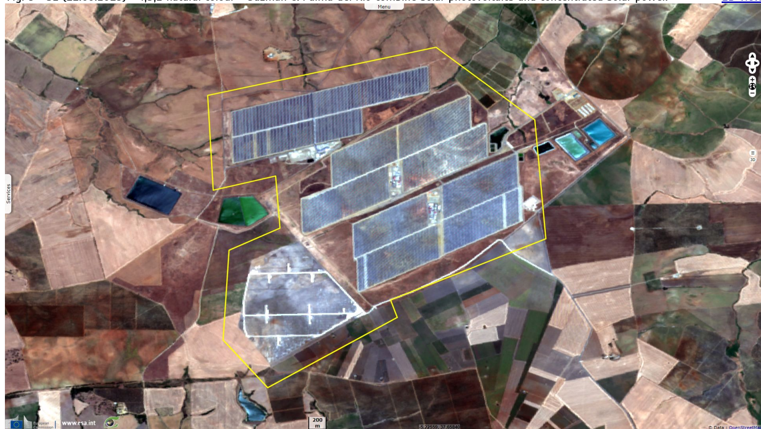
Fig. 9 - S2 (11.06.2019) - 4,3,2 natural colour - Guzman & Palma del Rio combine solar photovoltaics and concentrated solar power.
