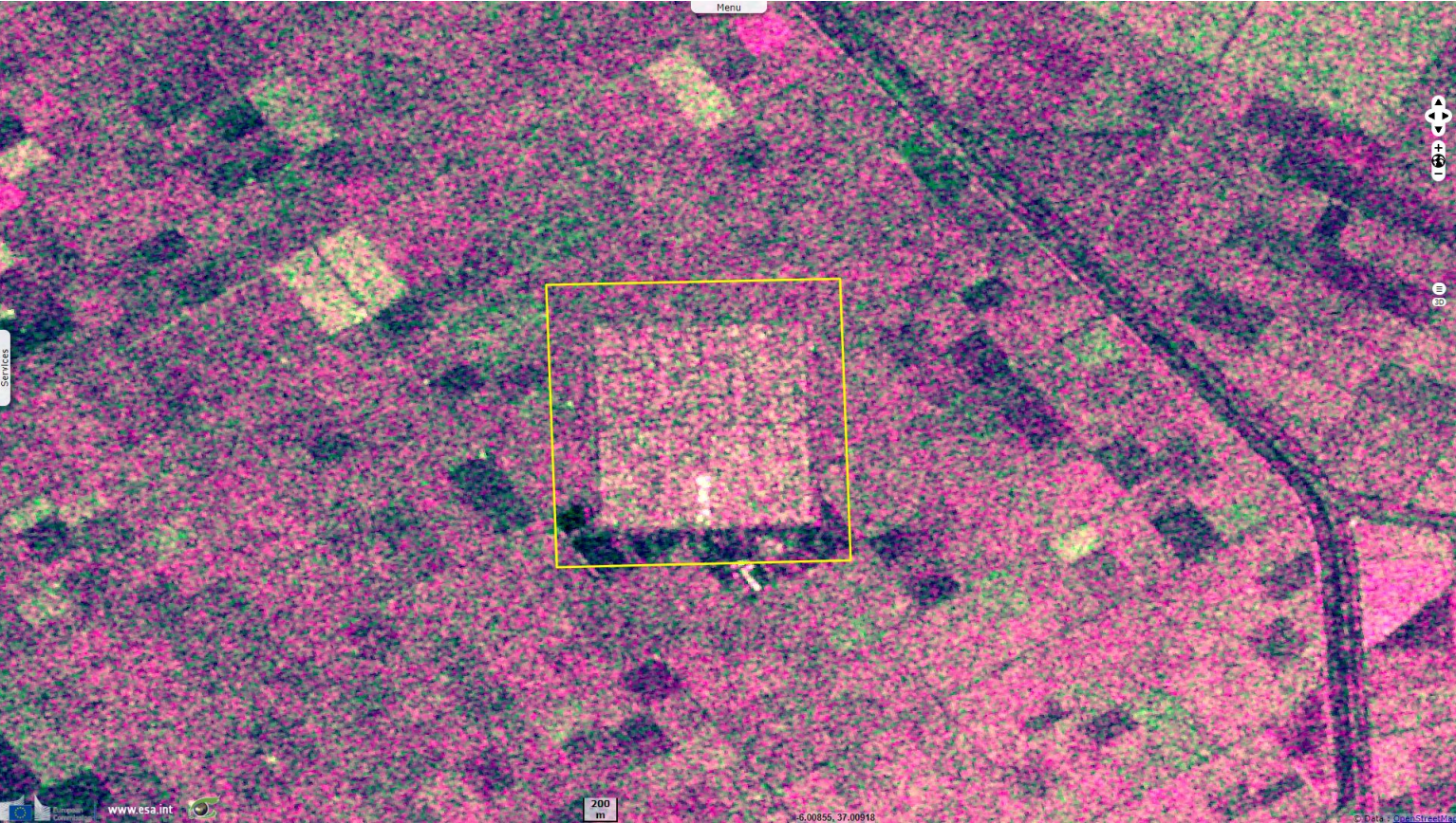
Fig. 14 - S1 (20.10.2019 18:18) - vv,vh,vv colour composite - South of Seville near the Guadalquivir, Lebrija-1 50 MW parabolic trough project. 2D view
