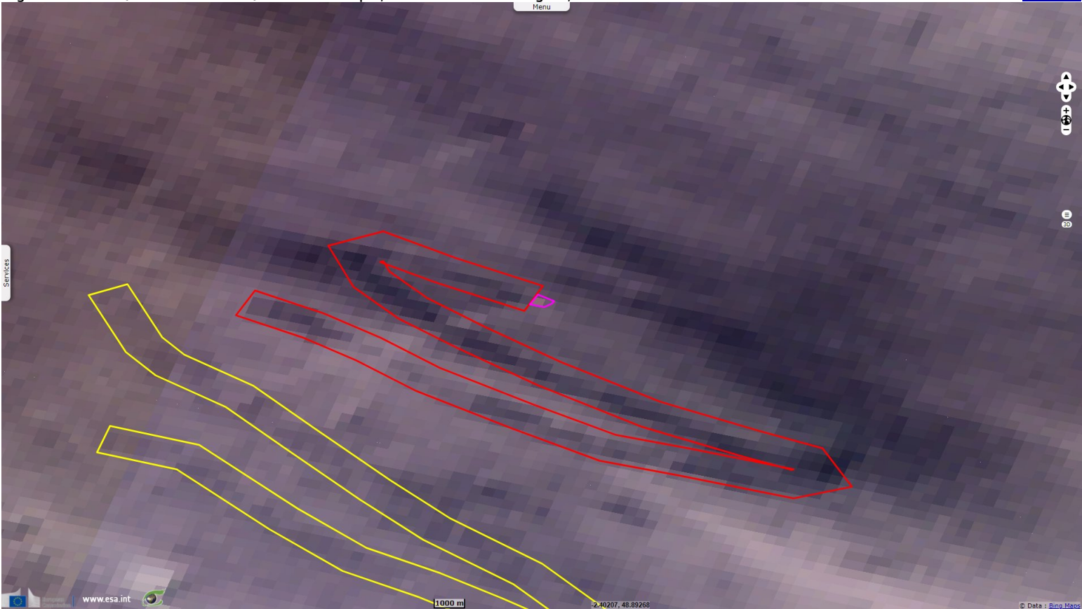
Fig. 4 - S3 OLCI (13.06.2021 10:56) - The same spill, not seen in the sun glint, can be found to be between 14h and 26h old.
