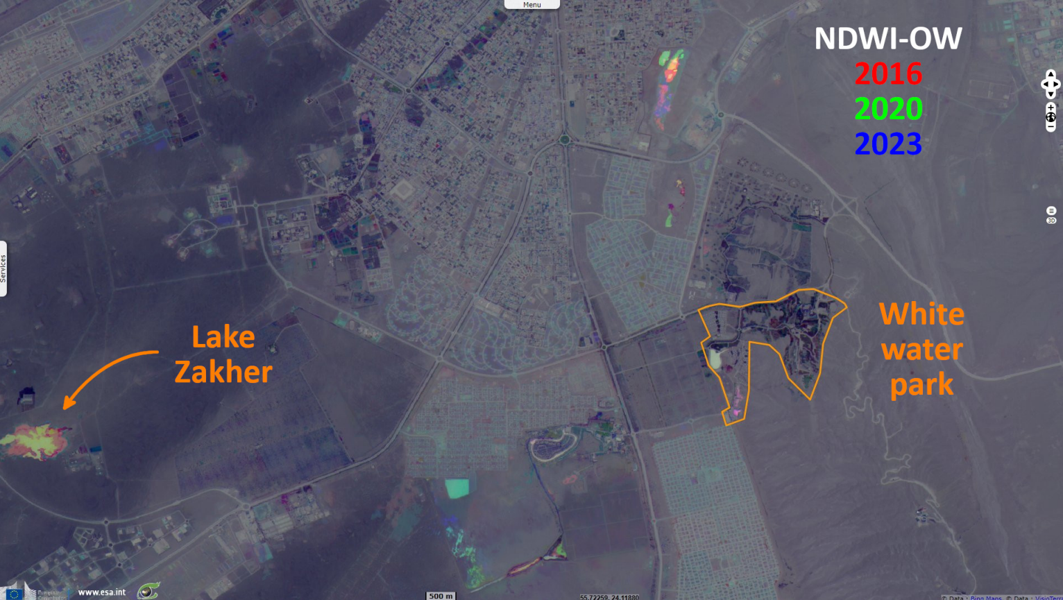
Fig. 2 - S2 (18.07.2016, 12.07.2020, 17.07.2023) - The Open Water index shows small changes along time in artificial water bodies.
