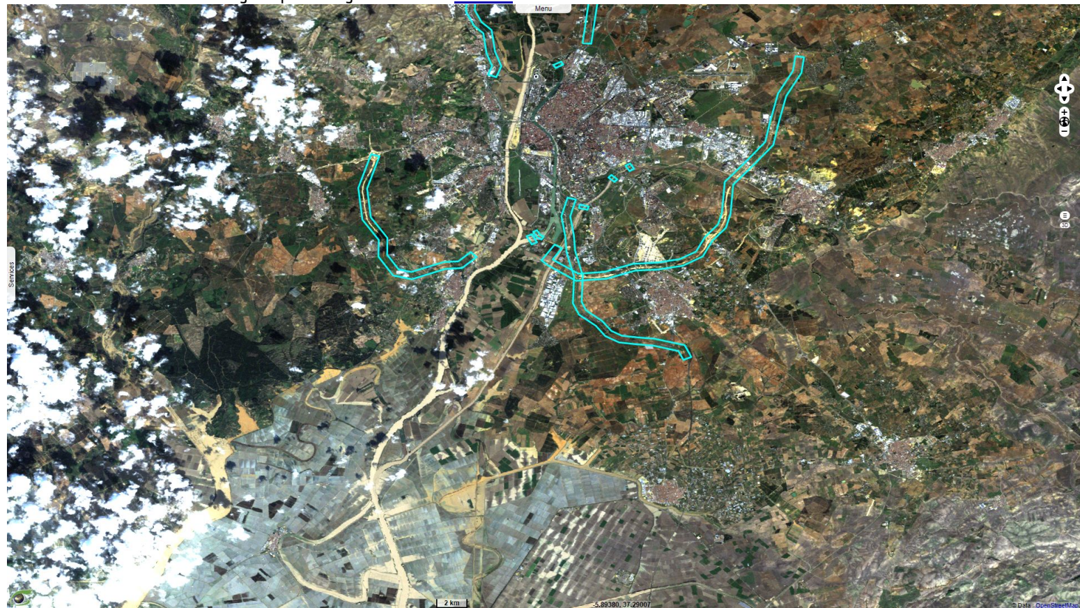
Fig. 13 - L5 (23.12.2010) - 3,2,1 natural colour - Flood of winter 2010-11, new roads & bridges are outlined in cyan. Infrastructure improvement such as the new river lock or its change of path mitigate the risk. 2D view
