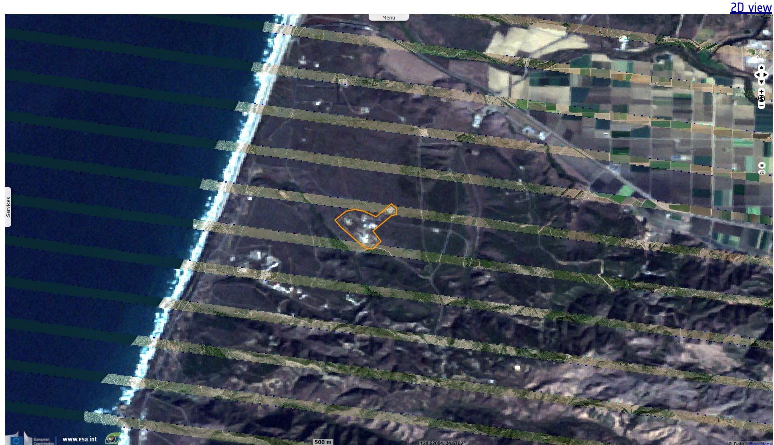
Fig. 3 - L7 (23.11.2020) - Landsat-7 was launched in 1999, its sensor has 6 30m optical bands, a 15m panchromatic & a 60m thermal IR. It has a 16-day cycle.
