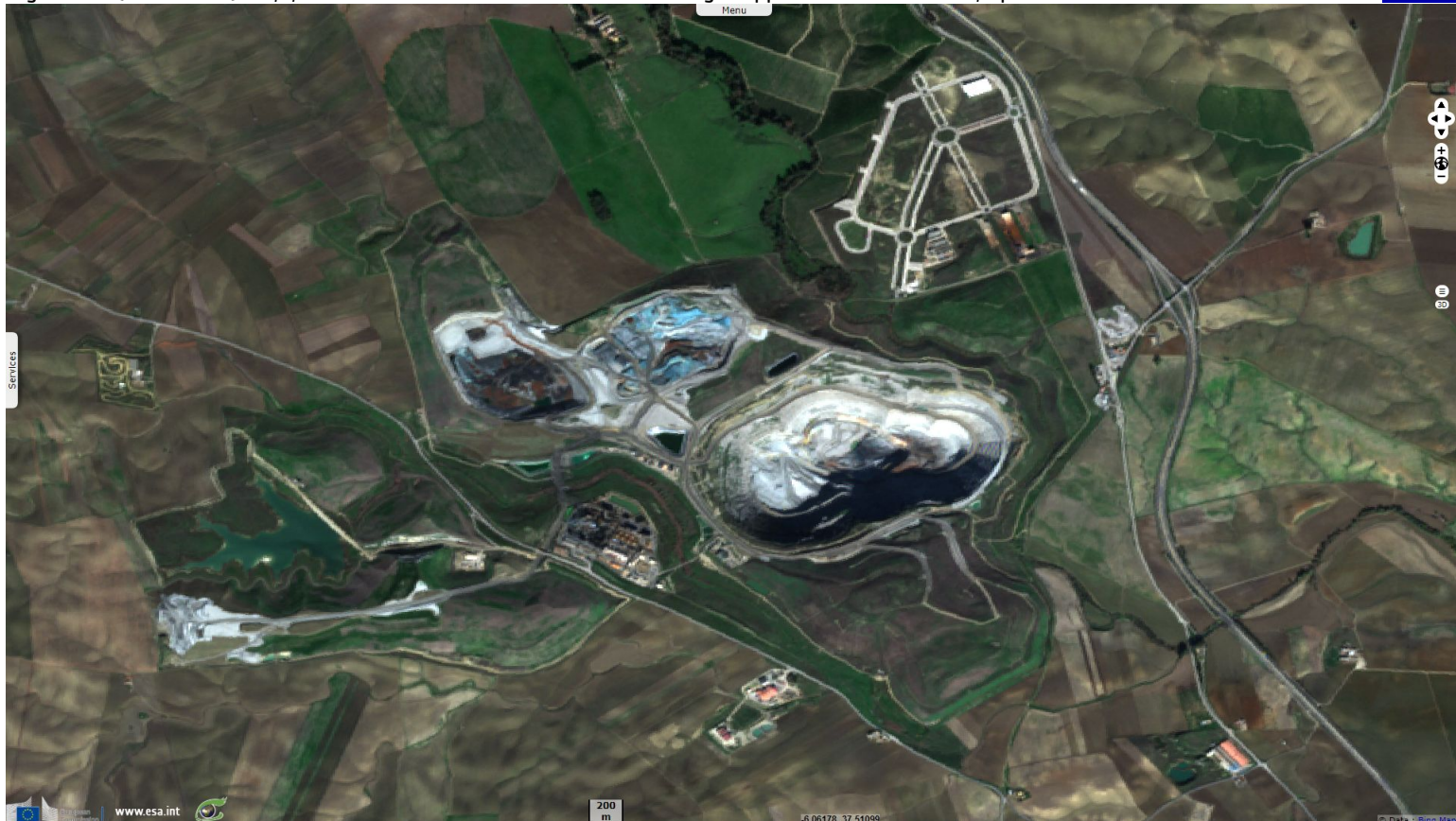
Fig. 2 - S2 (27.01.2019) - Various colours and layers show as a 1.3 km front in the north-west slope collapsed 300 m lower .
