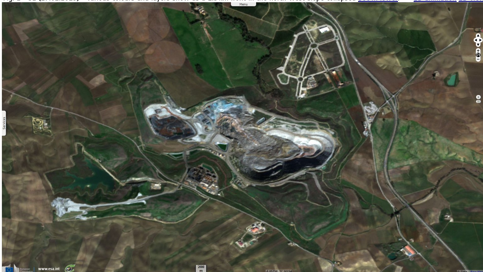
Fig. 2 - S2 (27.01.2019) - Various colours and layers show as a 1.3 km front in the north-west slope collapsed 300 m lower .
