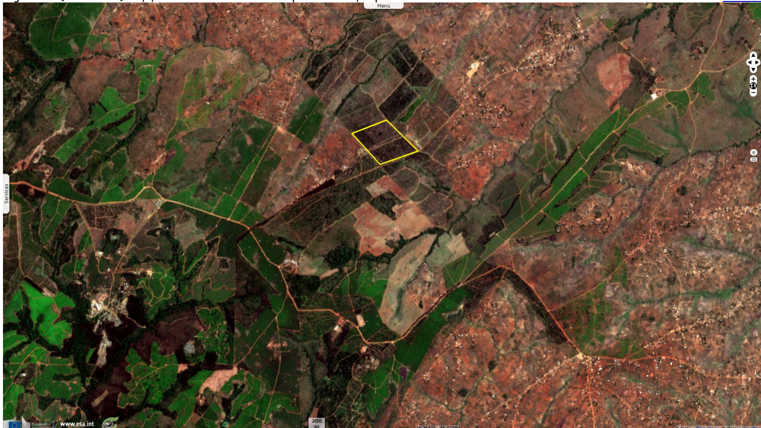
Fig. 2 - S2 [26.09.2018] - ndi(8,4) with colour map - Normalized Difference Vegetation Index of the same acquisition.
