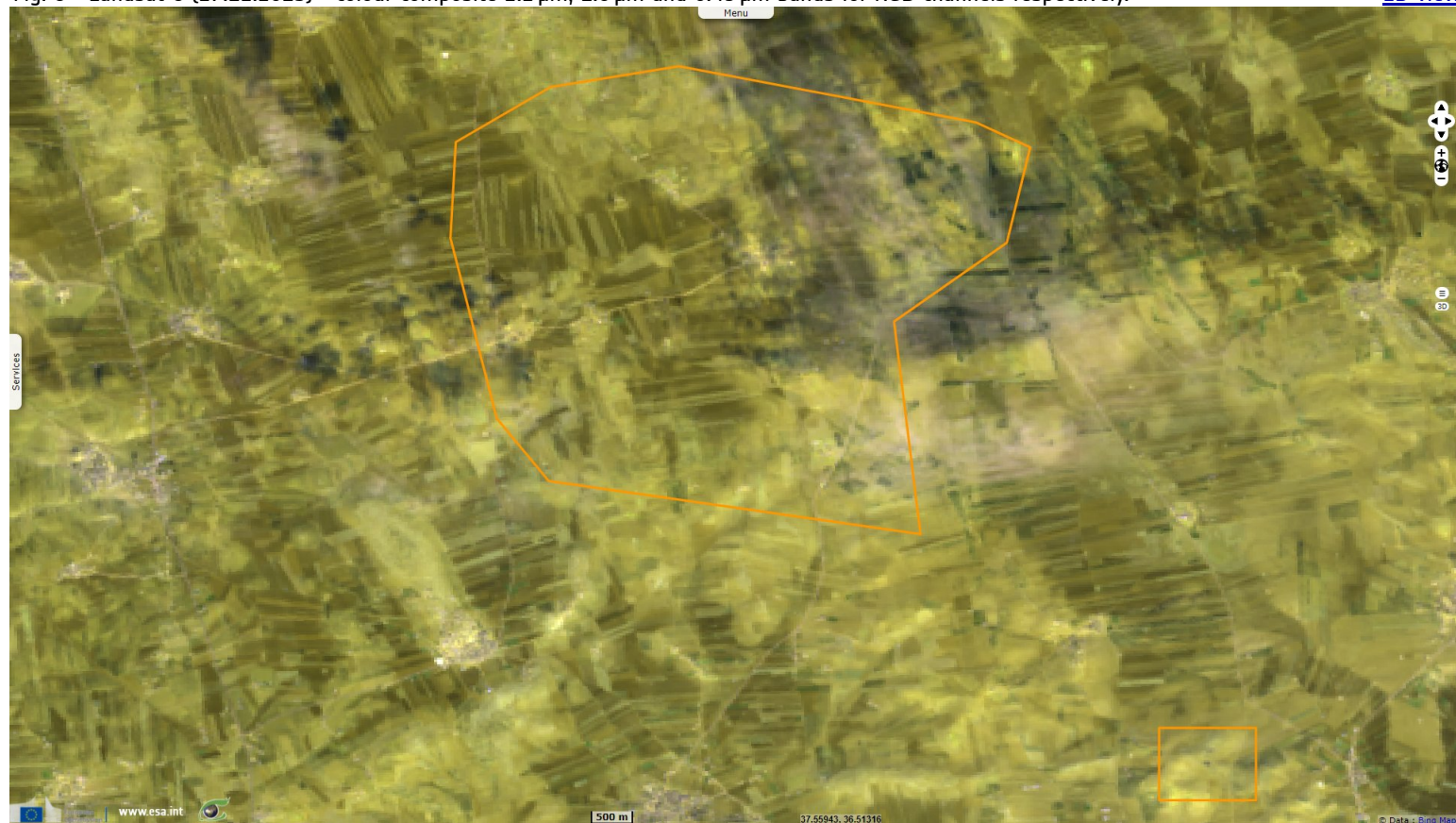
Fig. 8 - Landsat-8 (27.12.2013) - colour composite 2.2 \mu\text{m} , 1.6 \mu\text{m} and 0.49 \mu\text{m} bands for RGB channels respectively.
