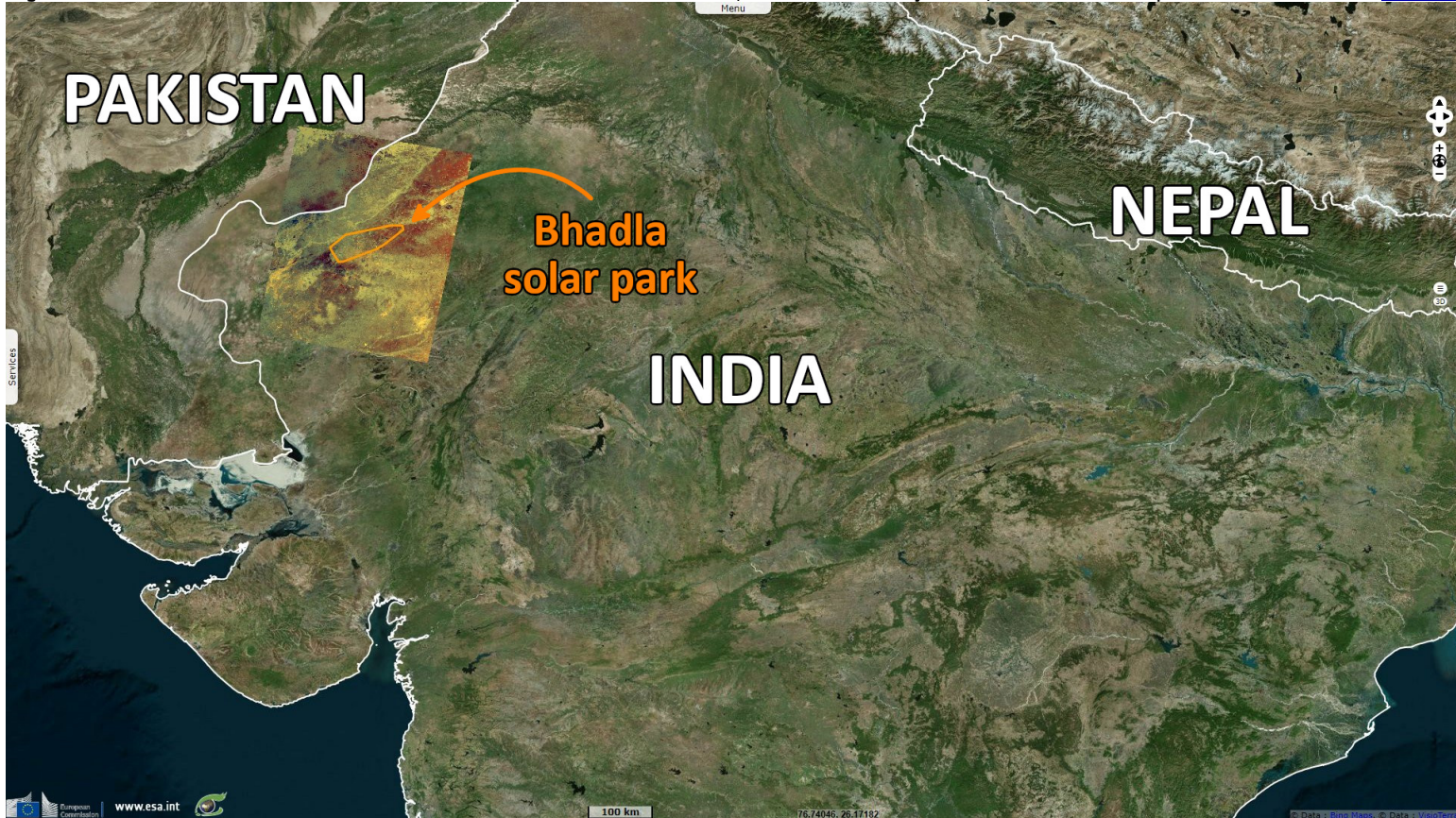
Fig. 2 - S2 (11.03.2023) - This is the largest solar park in the World with a surface of 5700 ha and a total capacity of 2245 MW. 3D view
