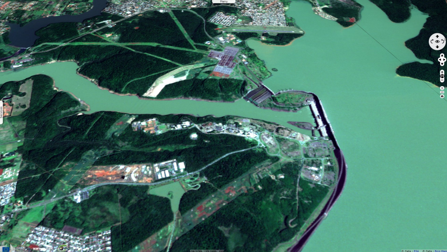
Fig. 4 - S2 (16.04.2016) - The dam is 196 m high, equivalent to a 65-story building. It is 8 km long, with a reservoir volume of 29 km³. 3D view
