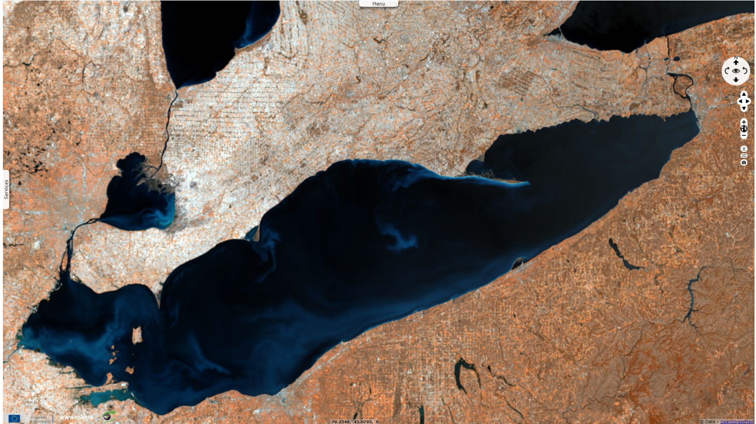
Fig. 8 - 30.04.2018 - 18,11,8 colour composite - The blooms show less reflectance in red edge & near infrared than in green. 3D view 3D animation
