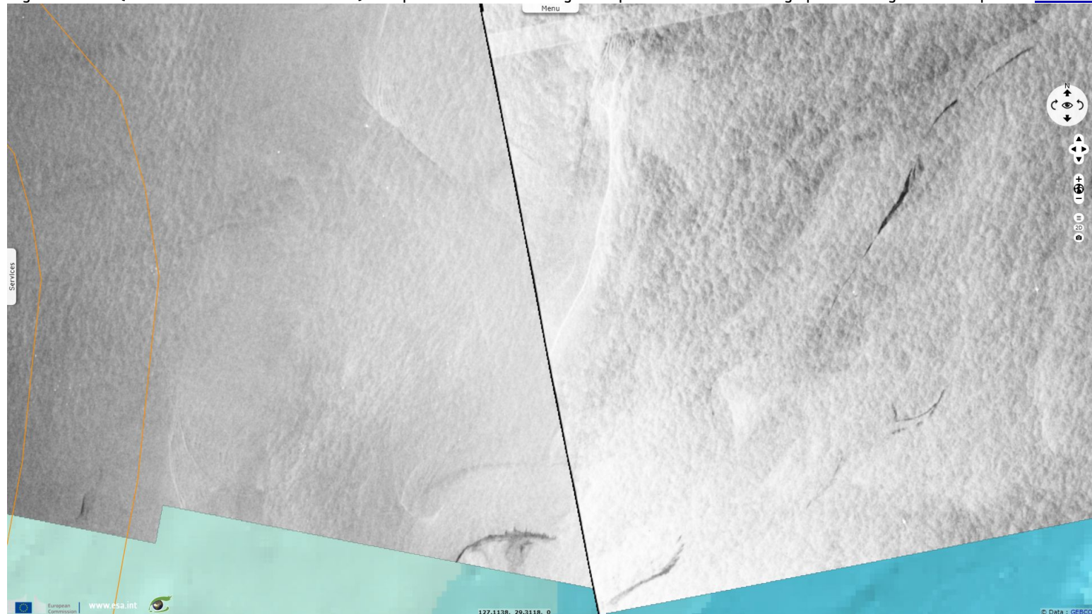
Fig. 8 - S1 IW (20.01.2018 09:28:53 & 21:33:37) - vv polarization with histogram equalization - 60+km long spills heading towards Japan. 3D view
