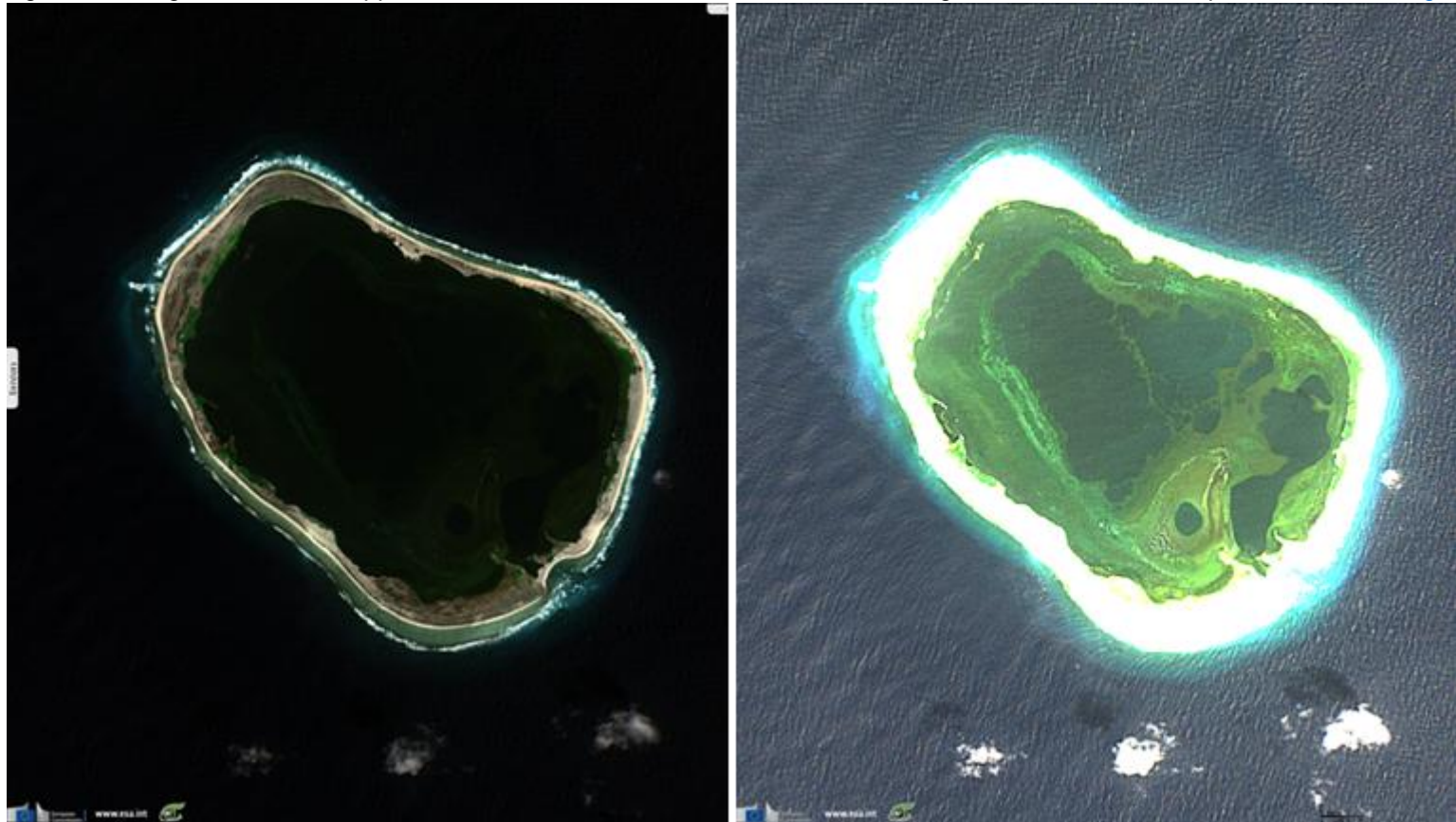
Fig. 4 - S2 image - 8-11-2 colour composite (left) - Normalised Difference Index between bands 2 and 5 (right). left right
