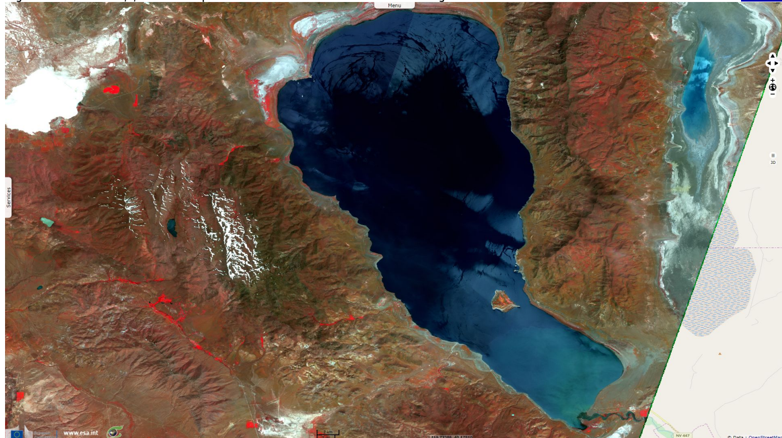
Fig. 3 - 10.05.2017 - 8,4,3 colour composite - The mouth of Truckee river & thin biogenic films north show low reflectance in Near InfraRed. 2D view
