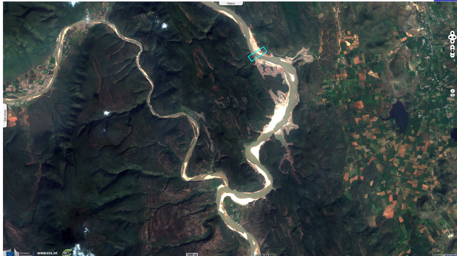
Fig. 4 - S2 (04.12.2021) - Optical view of the lake after the dam failure. The lake has emptied while the upstream waters are stronger than previously.
