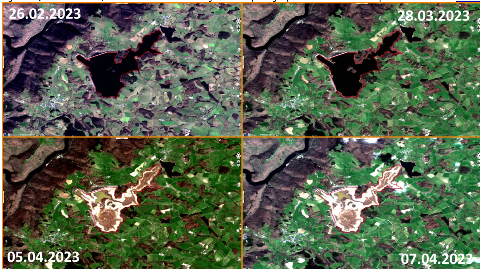
Fig. 2 - S2 [26.02 - 07.04.2023] - The reservoir of the second largest electricity storage system in France has been emptied for maintenance. 2D view
