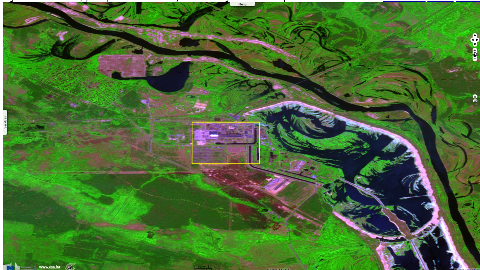
Fig. 4 - 2018.06.10 - ndi(8,4) with colour map - The decrease of vegetal cover is shown by the NDVI. 2D animation 2D view 2D view
