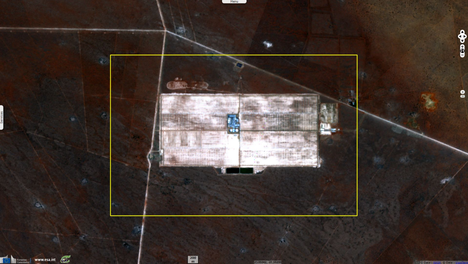
Fig. 5 - S2 (04.11.2019) - 4,3,2 natural colour - It has a capacity of 100 MW and full-load molten storage capacity of 4.5 hours. 2D view
