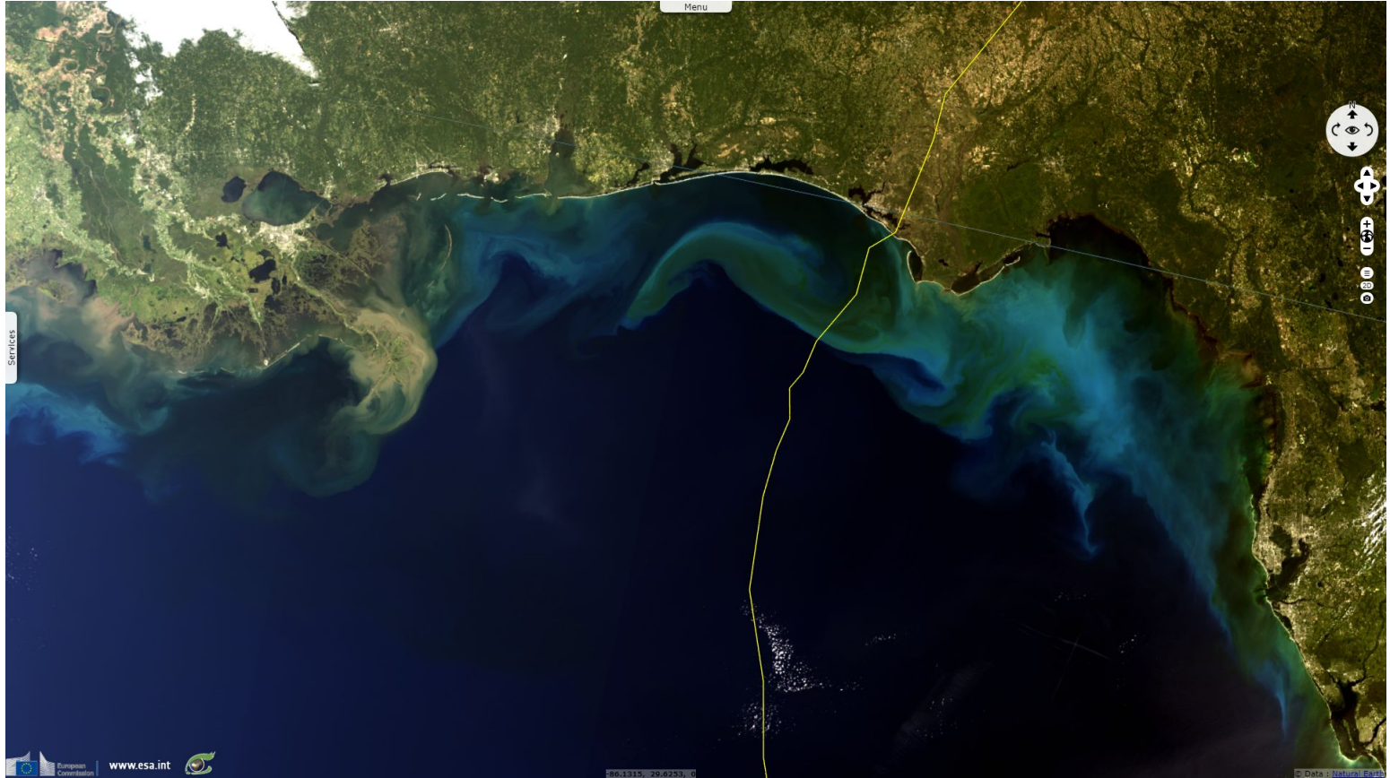
Fig. 5 - S3 OLCI (13.10.2018) - 7,6,4 colour composite - Heavy rainfalls increased runoff, sediment & plankton-friendly nutrients.
