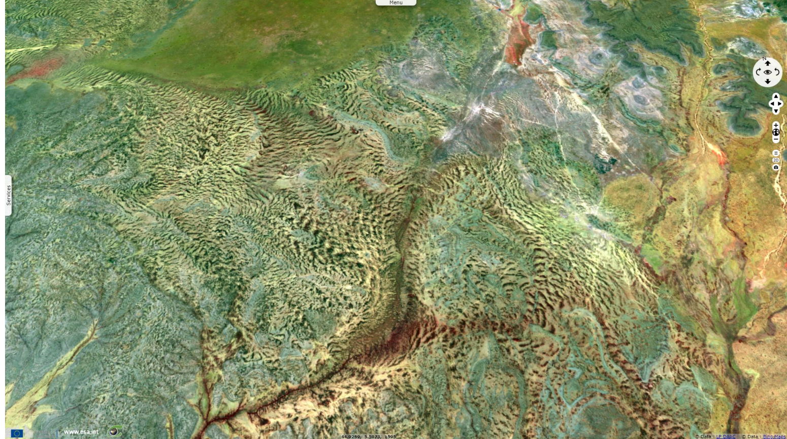
Fig. 6 - ndi(8,4) with colour map - NDVI of the same low slope area; separated by bare ground, the run roughly parallel to contour lines. 3D view
