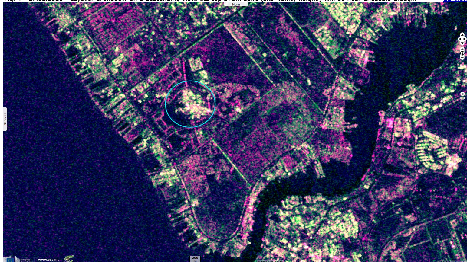
Fig. 4 - 17.01.2020 - Layover & shadow on a descending view. Its top 370m spire (aka 'vanity height') will be near-unusable though. 2D view
