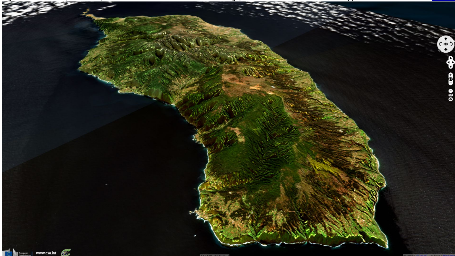
Fig. 2 - S2 MSI L2A (13.02.2019) - The contrast is increased in the L2A image, but discontinuities between tiles appear.
