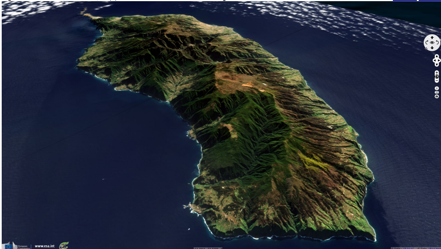
Fig. 2 - S2 MSI L2A (13.02.2019) - The contrast is increased in the L2A image, but discontinuities between tiles appear.
