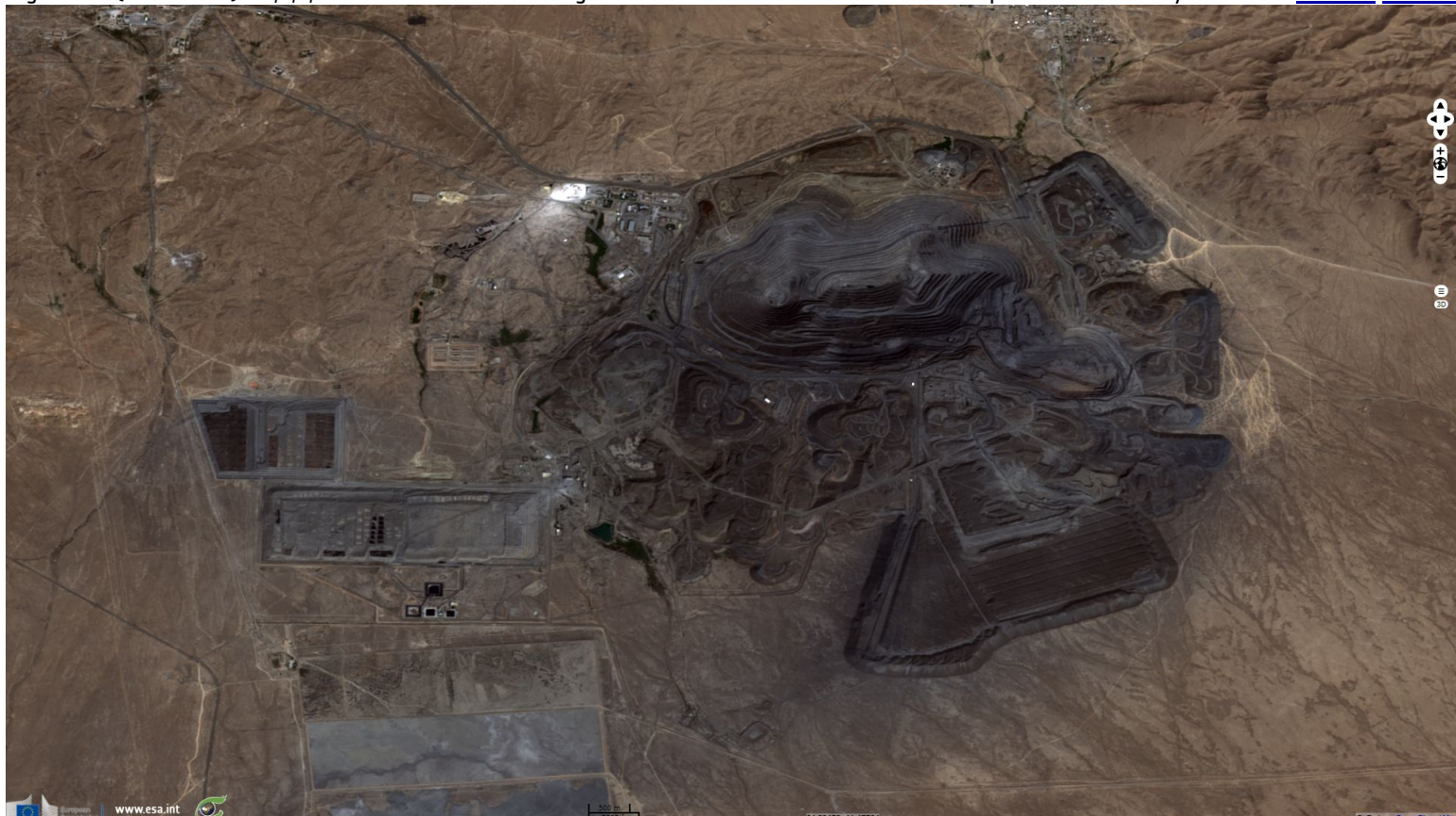
Fig. 2 - S1 (28.03.2018) - vv,vh,ndi(vh,vv) colour composite - The pits depth shows thanks to the radar shadows & foreshortening. 2D view 3D view
